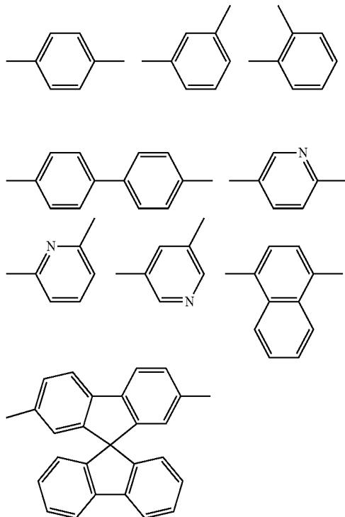
In Formula (201) described above,  $\text{Ar}^1$  is an arylene group having 6 to 60 carbon atoms which may have a substituent, a pyridinylene group which may have a substituent or a quinolinylene group which may have a substituent. Substituents for the respective groups represented by  $\text{Ar}^1$  and  $\text{Ar}^2$  each are the same as explained for R described above.
