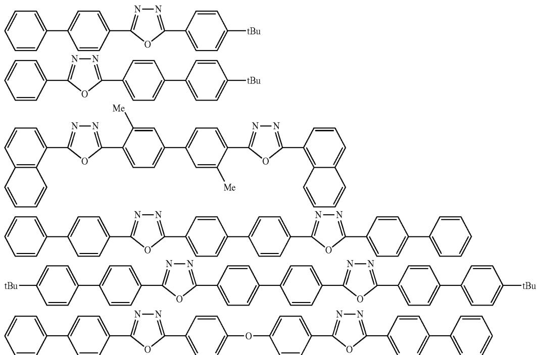
The nitrogen-containing heterocyclic derivative includes nitrogen-containing compounds which are nitrogen-containing heterocyclic derivatives comprising organic compounds represented by the following formulas and which are not metal complexes. They include, for example, five-membered rings or six-membered rings having a skeleton represented by (A) and compounds having a structure represented by (B).
