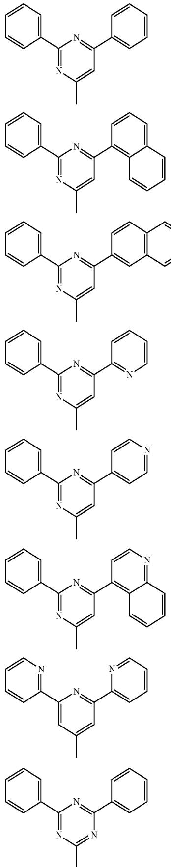
In the respective formulas described above, R is an aryl group having 6 to 40 carbon atoms, a heteroaryl group having 3 to 40 carbon atoms, an alkyl group having 1 to 20 carbon atoms or an alkoxy group having 1 to 20 carbon atoms; n is an integer of 0 to 5, and when n is an integer of 2 or more, plural R may be the same as or different from each other.
