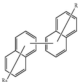
Phosphorescent OLEDs prepared by using the host material represented by Formula (2) described above, and a phosphorescent material exhibit high efficiency and long lifetime. Preferably, the phosphorescent material is a red phosphorescent material.
