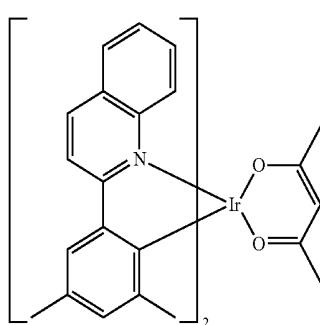
In another embodiment, the phosphorescent emitter material comprises a metal complex, and the metal complex comprises a metal atom selected from Ir, Pt, Os, Au, Cu, Re and Ru and a ligand. In yet another embodiment the metal complex has an ortho-metal bond. The metal atom is preferably Ir.
