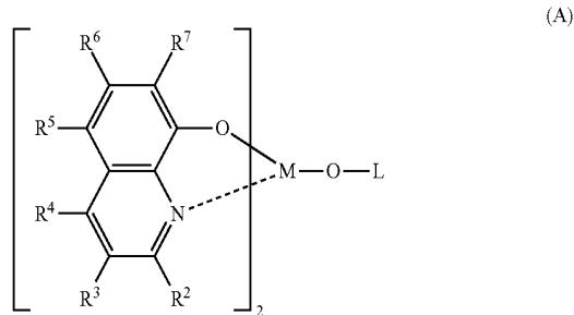
R<sup>2</sup> to R<sup>7</sup> each are independently a hydrogen atom, a halogen atom, an oxy group, an amino group, a hydrocarbon group having 1 to 40 carbon atoms, an alkoxy group, an aryloxy group, an alkoxy carbonyl group or a heterocyclic group, and they may be substituted.
